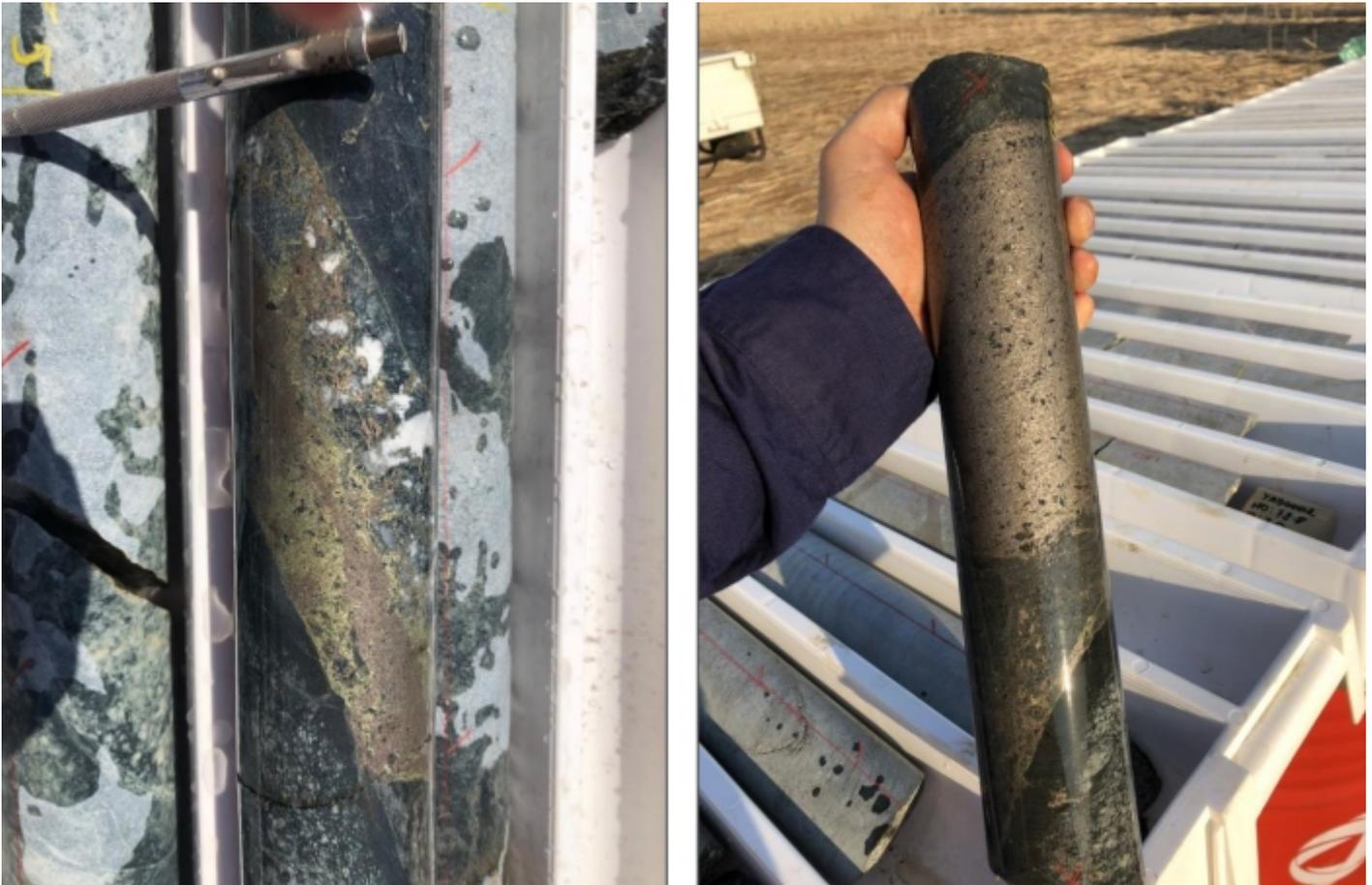
Left: Chalcopyrite and pyrrhotite mineralisation in hole YAD0001. Right: Massive pyrrhotite mineralisation with minor pentlandite in hole YAD0002.
